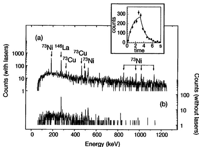
FIG. 1. Part of the  $\gamma$  spectrum at mass 73 obtained (a) with and (b) without laser light irradiating the gas cell. The integrated proton beam dose was  $1.6 \times 10^5$  and  $5.7 \times 10^4 \mu\text{C}$ , respectively. The time evolution of the  $\gamma$  intensity attributed to the decay of  $^{73}\text{Ni}$  is given in the inset.
