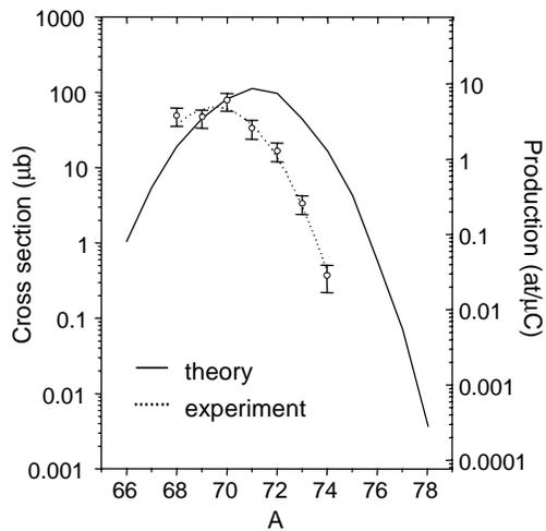
FIG. 2. Comparison of experimental production yields for  $^{68-74}\text{Ni}$  and cross section calculations for 30 MeV protons on  $^{238}\text{U}$  [22]. A possible  $\beta$ -delayed neutron branch in  $^{74}\text{Ni}$  is not taken into account.
